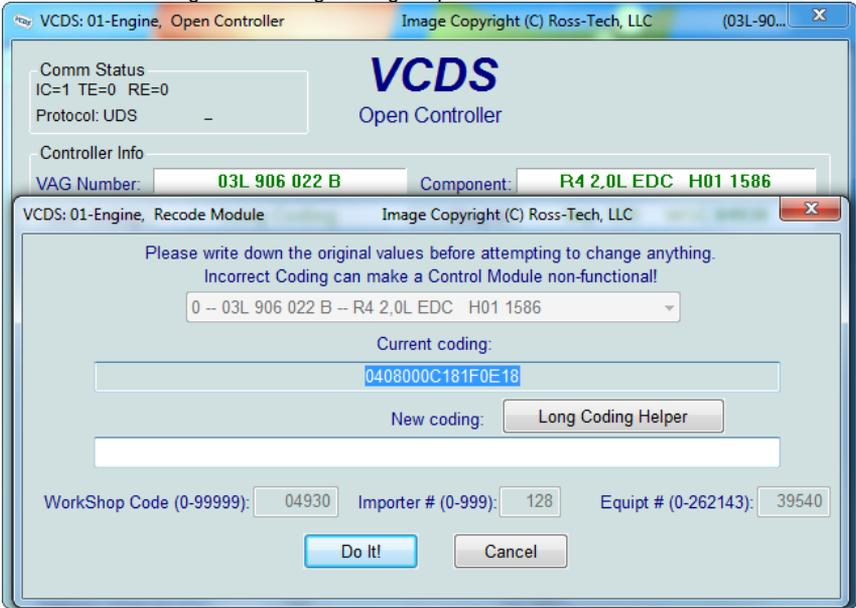
**Long Coding Helper** is used with applications such as Niels Ezerman's excellent LCode.exe (included with the latest distribution of VCDS). Click on each of the Byte numbers in row 3) and you'll see the selectable options in row 4). They can be individual checkboxes as shown below. Check or Un-check the boxes for the desired results. Example: "Adaptive Cruise Control (ACC) installed".
